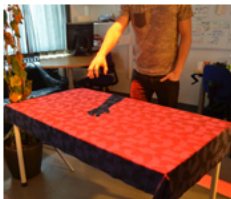
Figure 54. Colour Ball prototype. The rotation of the wrist manipulates the red, green, and blue colour parameters
