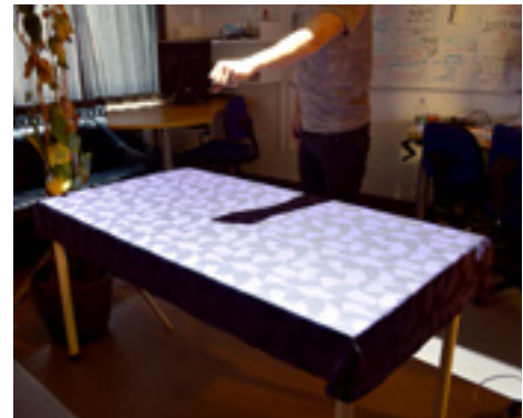
Figure 44. One Arm Brightness prototype. Arm is moved up and down to adjust brightness. A grab pose is one option for interaction
