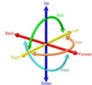
Figure 23. The 6 degrees of freedom in 3D space, here illustrating arm moment
