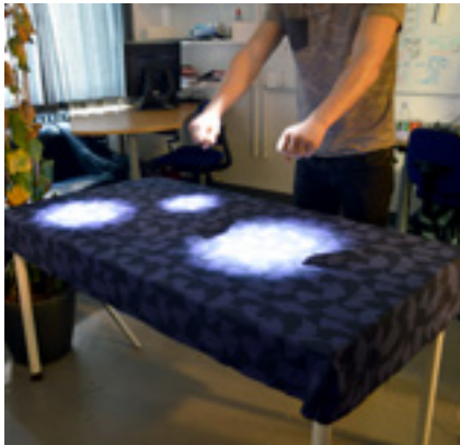
Figure 61. Tangible Lights prototype. Multiple spotlights can be created, grabbed, moved, scaled, and removed
