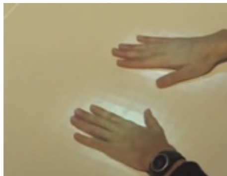
Figure 18. Video frame from the SmartSkin project by Rekimoto (2002). Surface gestures are tracked using capacitive sensing in the surface, and graphics are projected from above
